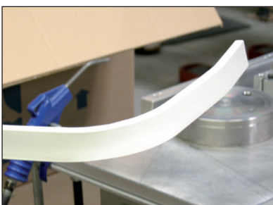
Once cooled, the moulding will retain the shape it was fixed in.
