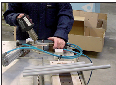
Heat gently using a hot air gun before bending to the required shape.
