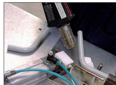
Apply heat evenly over a large area to achieve a smooth, even bend.
